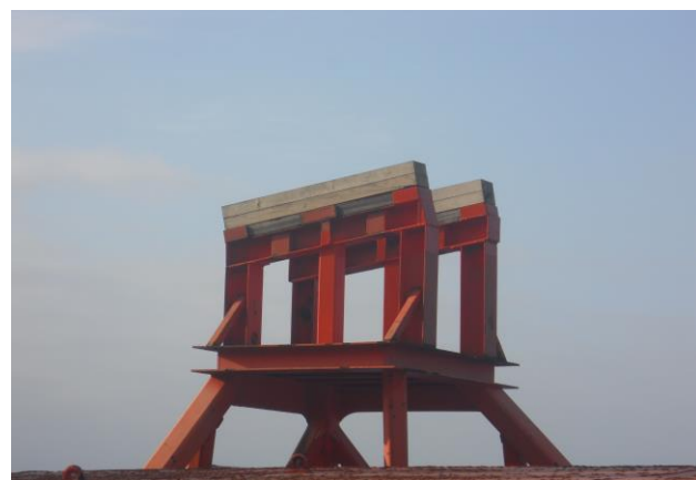
CRANE REST CHOCK AS NORMALLY SITUATED.
