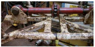
When the fully closed position was re-created with the VBC orientated over the filler cap at the onshore test facility the drum was deformed With the distortion of the drum, the clamps not being under the rim, the weight of the drum and the motion of the lift meant the drum worked its way free of the clamp.
