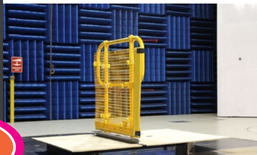
Wind Tunnel testing to determine C_{fig} value: Mesh Panel only
