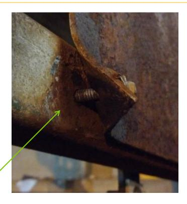
Singular remaining bolt as was found when load was landed on the rig.
