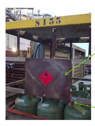
A review of other gas racks of the same design (S133, also received on the same shipment) revealed that various plates were not installed with all bolts as per design and these were only installed with 4 bolts rather than the 6 on R010.
