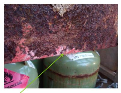
A review of the plate installed at the opposite side of the same rack (R010) revealed that this was also damaged and notable 1 of the 6 bolts installed had been sheared off at some point due to contact with something painted red. This plate remained securely fixed to the rack.
