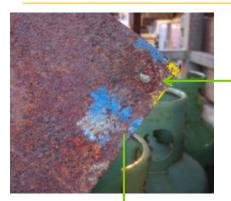
Fresh blue paint evident on top corner (which suggests that rack contacted other cargo or indeed the boat which is also blue, during the transit from Den Helder)
