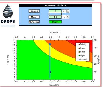
From DROP's Calculator mass alone would be enough to cause injury but shape is such that injury could be potentially fatal.
