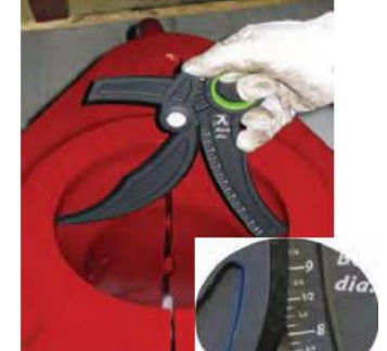
Measure elevator TJ-Bore (ID) with 2-point measurement. Readout 8. 1/4".
