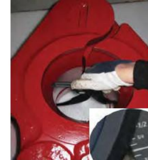
Measure elevator bore (ID) with 2-point measurement. Readout 6. 1/8".
