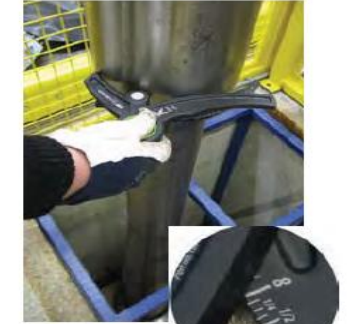
Measure pipe TJ-Diameter (OD) with 3-point measurement. Readout 8". The tool joint matches with the bore.
