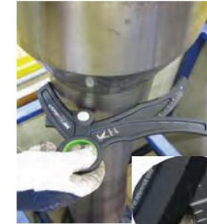
Measure pipe body (OD) with 3-point measurement. Readout 6". The pipe matches with the bore.
