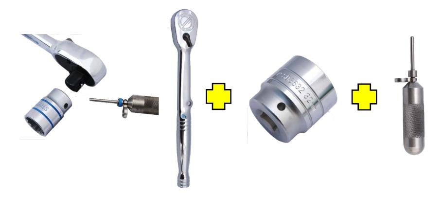
Using a pin locking mechanism prevents the tool coming separating.
