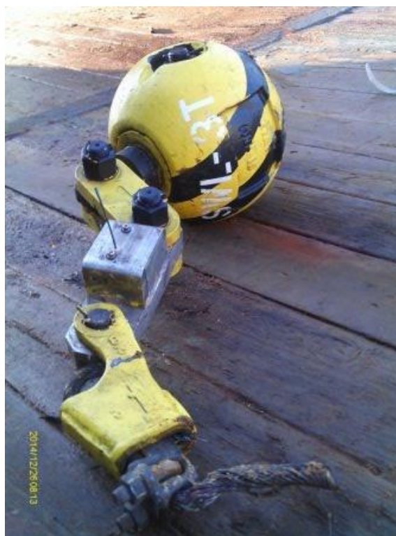
Figure: crane block that fell
