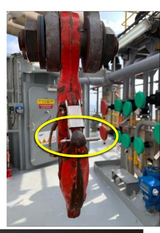
The rigger onboard the installation did report the defect however they carried on using the crane and failed to check if the gate was closed and locking pin was inserted.
