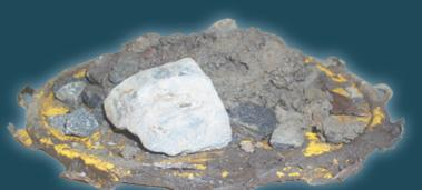
These are large (and heavy) lumps of rust from the pocket or substructure
