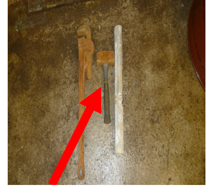
2lb Mash Hammer and Scaffold Pole that could have been potentially a dropped object
