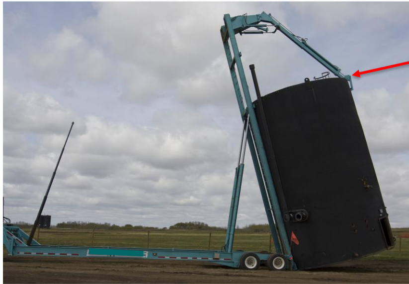
Example of a tank cradle arm with the bracket intact
