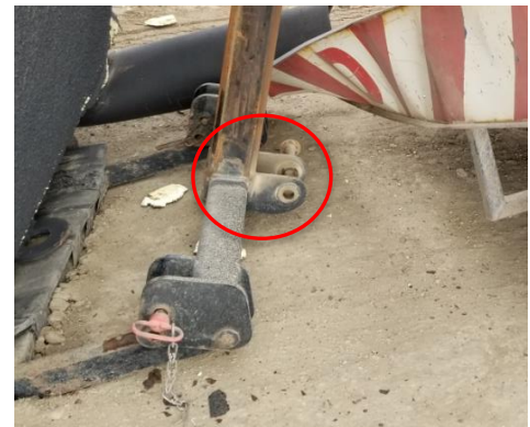
Close-up of the failed bracket with the Main mast pin out of position
