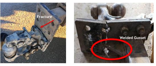
THE HITCH WAS RELOCATED TO THE UPPER MOUNTING POSITION AS EMERGENCY MEASURE TO REMOVE THE COMPRESSOR FROM THE HIGHWAY.
