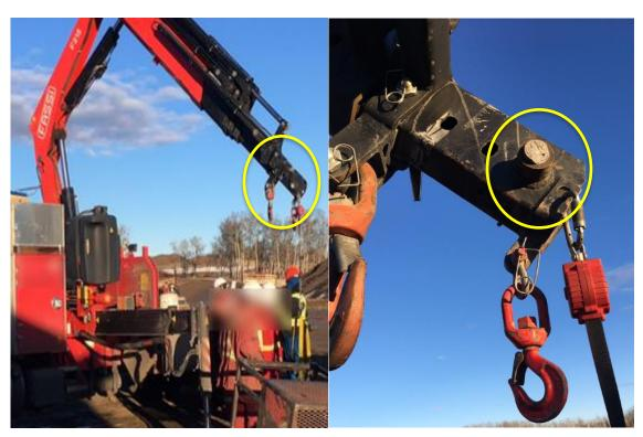
CIRCLE HIGHLIGHTS SHEARED PIN LOCATED. SHEARED PIN ON TOP OF KNUCKLEBOOM.
