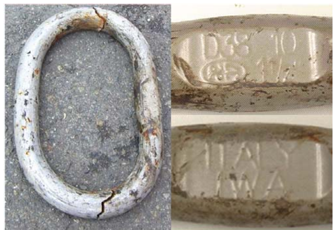
Cracked masterlink Manufacturer: Weissenfels
